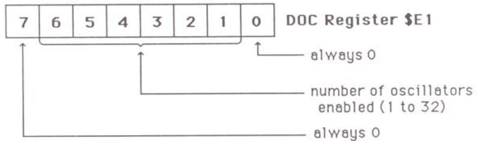
Note that the number of enabled oscillators affects the rate at which the DOC scans the oscillator wavetables. The more oscillators are enabled, the slower the rate. To simplify calculations, the GS sound tools enable all 32 oscillators.
