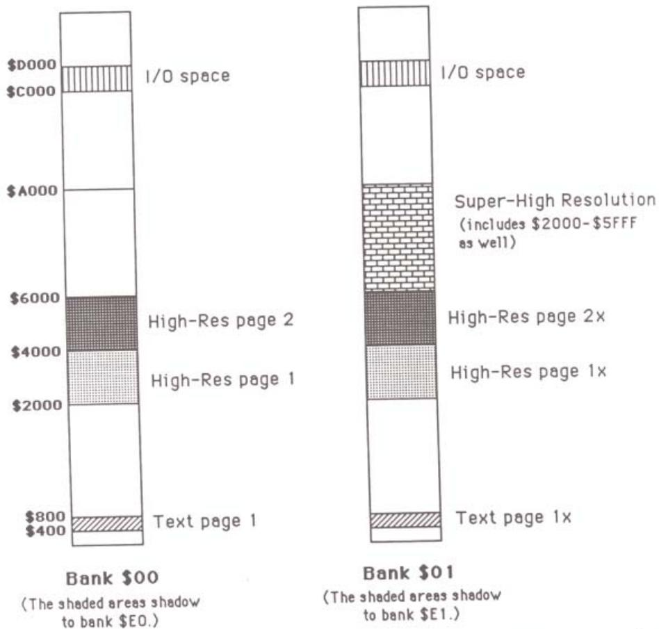
NOTE: Text page 2 (\$800-\$BFF) is shadowed using software techniques if Alternate Display Mode is On.
