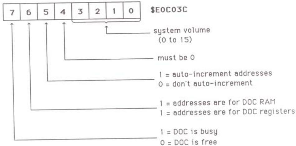
Bit 7 is a status bit that indicates whether the DOC is ready to respond to read and write operations. It is ready only if this bit is 0.
