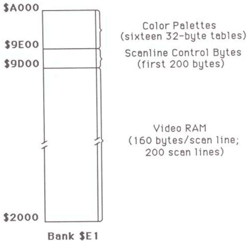
NOTE: Locations \$2000—\$9FFF in bank \$01 shadow to this bank if shadowing is enabled.
