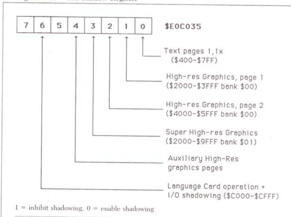
**NOTE:** Bit 4 works in conjunction with bits 1 and 2. If bit 1 is clear, the space from \$2000-\$3FFF in bank \$00 is shadowed to bank \$E0; if bit 4 is also clear, the same space in bank \$01 is also shadowed (to bank \$E1). Similarly, if bit 2 is clear, clearing bit 4 enables shadowing from \$4000-\$5FFF in bank \$01 (to bank \$E1) as well as the same locations in bank \$00 (to bank \$E0).
