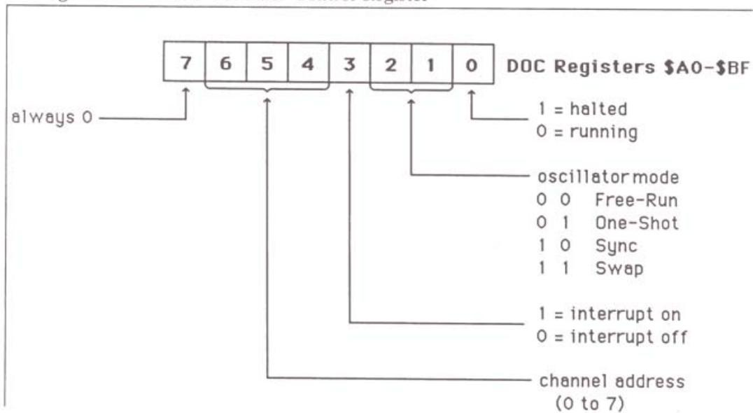
interrupts are enabled, the oscillator mode, and whether the oscillator has been halted or is playing.
