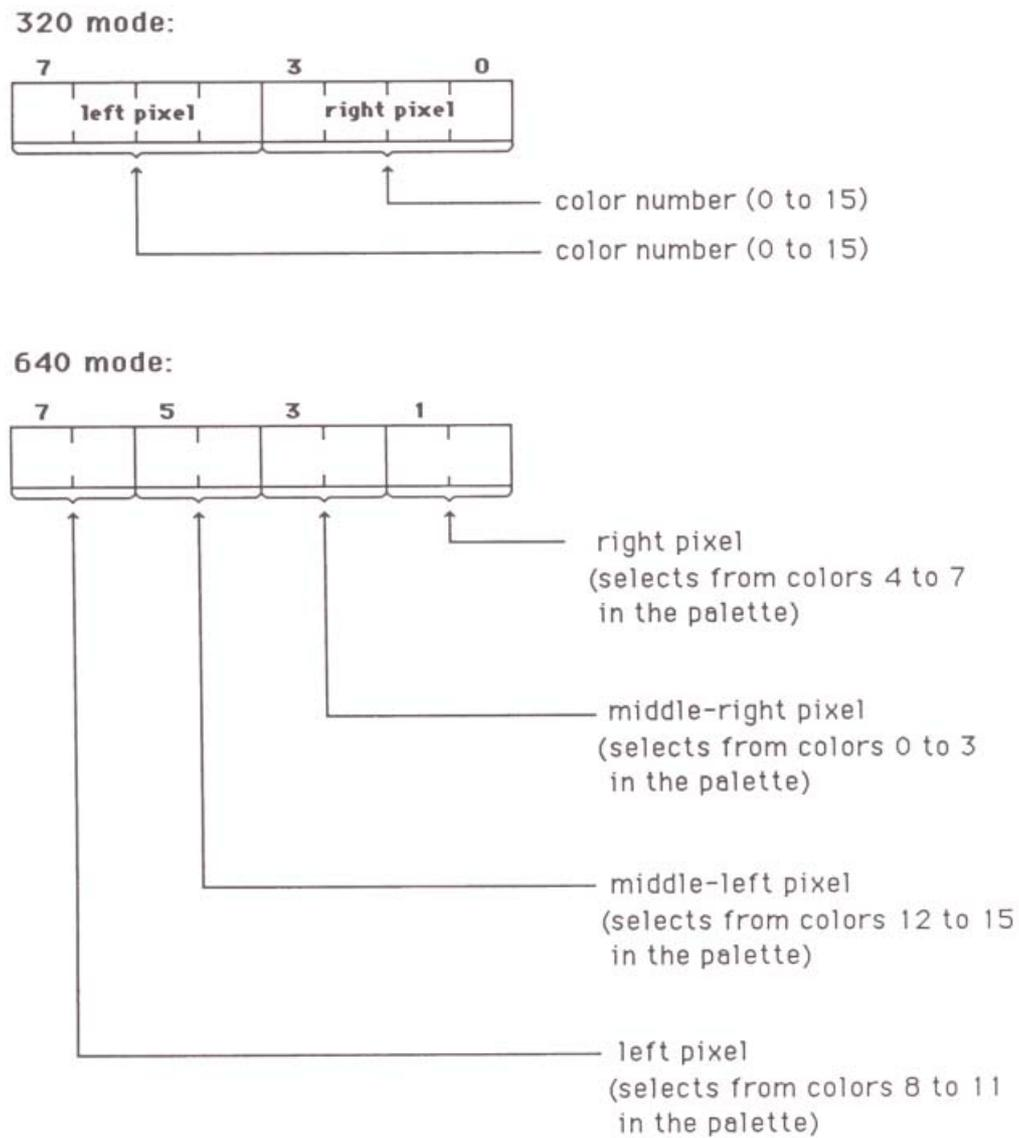
Figure 6-4. The Format of a Scanline Control Byte
